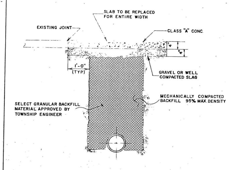
BACKFILL SHALL BE PLACED IN 6" LAYERS AND EACH LAYER COMPACTED BY VIBRATOR TAMPER, MACHINE TAMPER OR OTHER SUITABLE EQUIPMENT.
